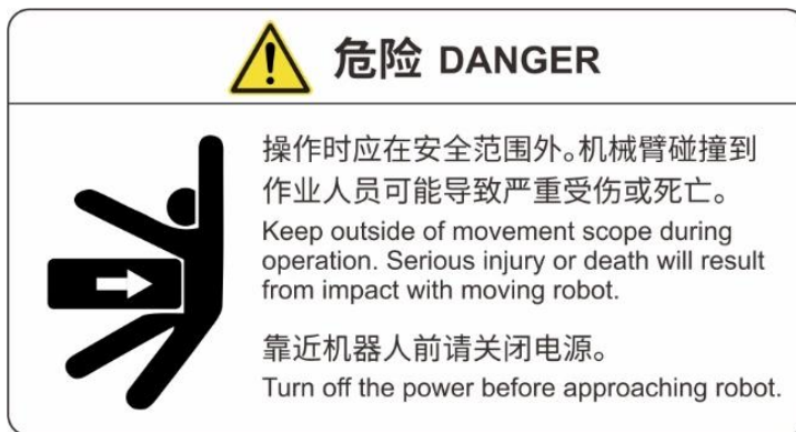
Figure 2- 5 Hazard warning label
