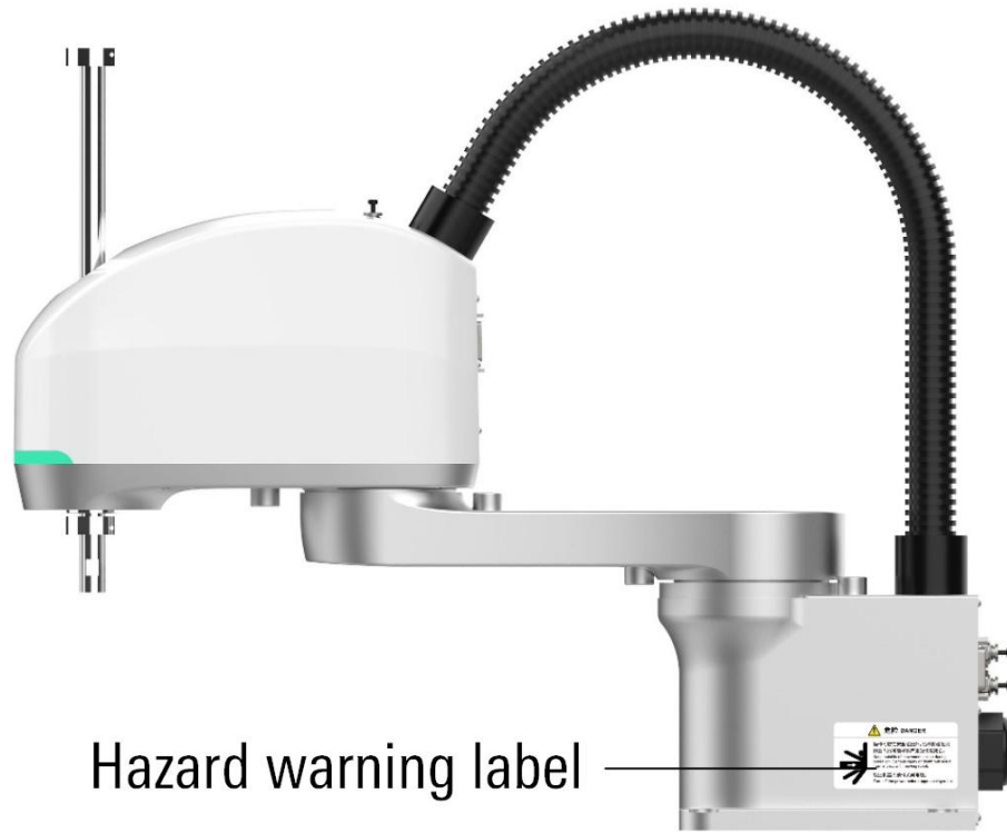
Figure 2-6 manipulator hazard warning label location diagram
