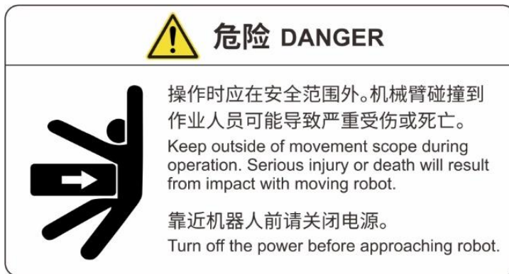
Figure 2- 5 Hazard warning label
