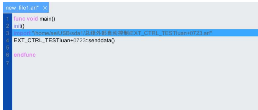
Figure 5-49 Subprogram is inserted along with its path (if it is not in the same path as the main program)
