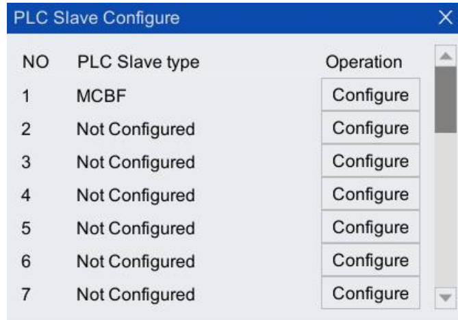
Figure 8-19 "PLC Slave Configuration" interface
