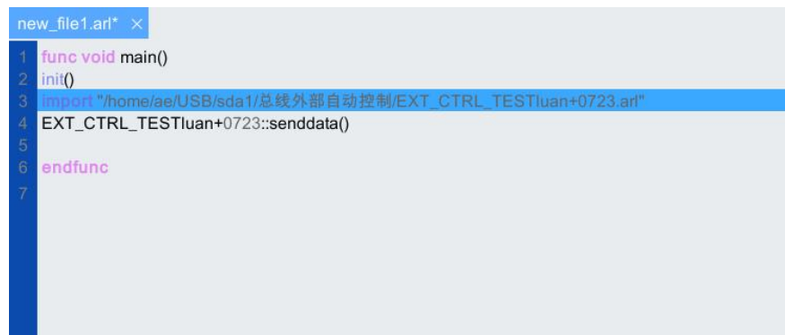
Figure 5-56 Subprogram is inserted along with its path (if it is not in the same path as the main program)
