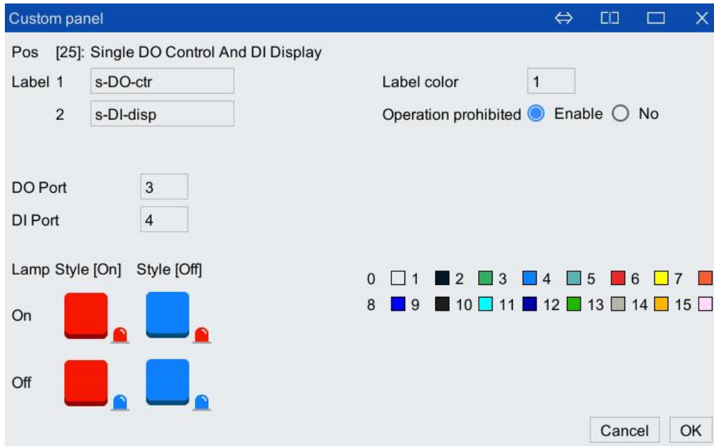
Figure 6-93 "Single DO control and DI display" Setting interface
