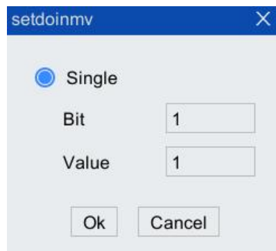
Figure 5-43 The "setdoimv" instruction configuration interface
