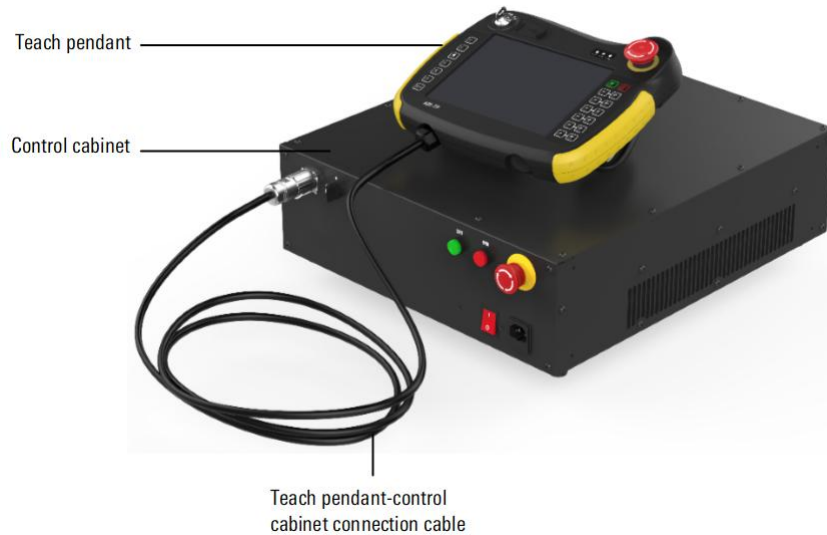
Figure 2-1 Where and how to place the robot teach pendant
