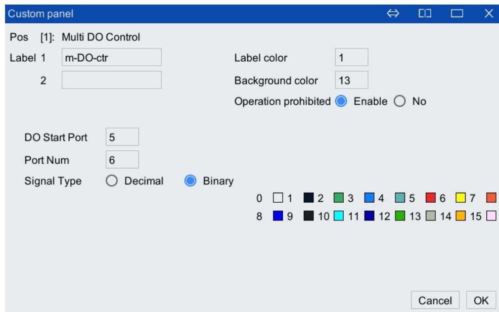
Figure 6-96 "Multi DO control" setting interface
