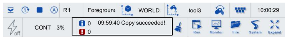
Figure 2-13 Teach pendant "message bar" alarm
